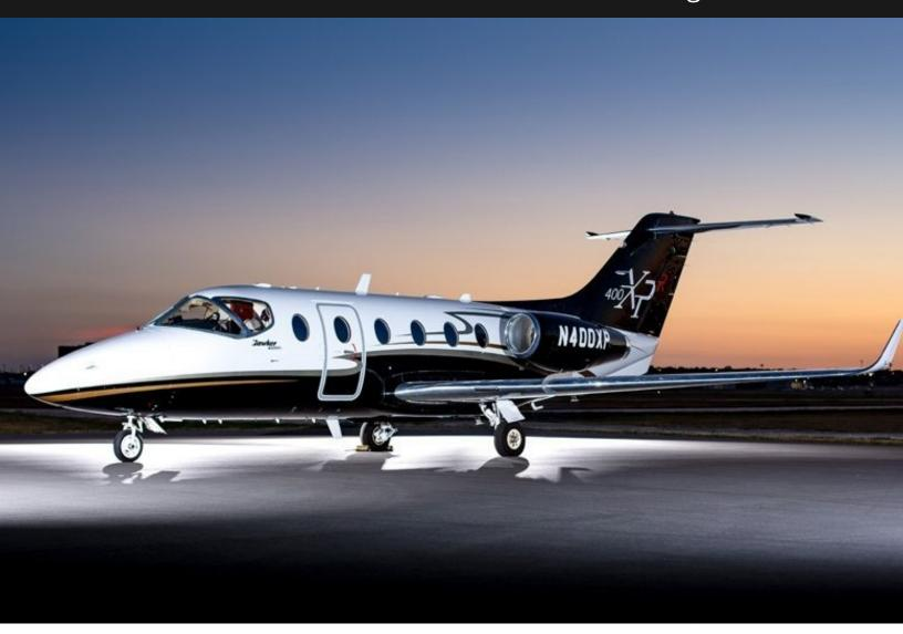
Transformation of the 400XPR entailed upgrading the customer's baseline Hawker 400XP with new Hawker winglets, Williams FJ44 engines. The full Hawker 400XPR package, which includes the winglets and new engines, provides a 33-percent increase in range, to 2,160 nm with four passengers, improvements in runway and hot/high performance and the ability to climb direct to FL450 in 19 minutes at max takeoff weight.
