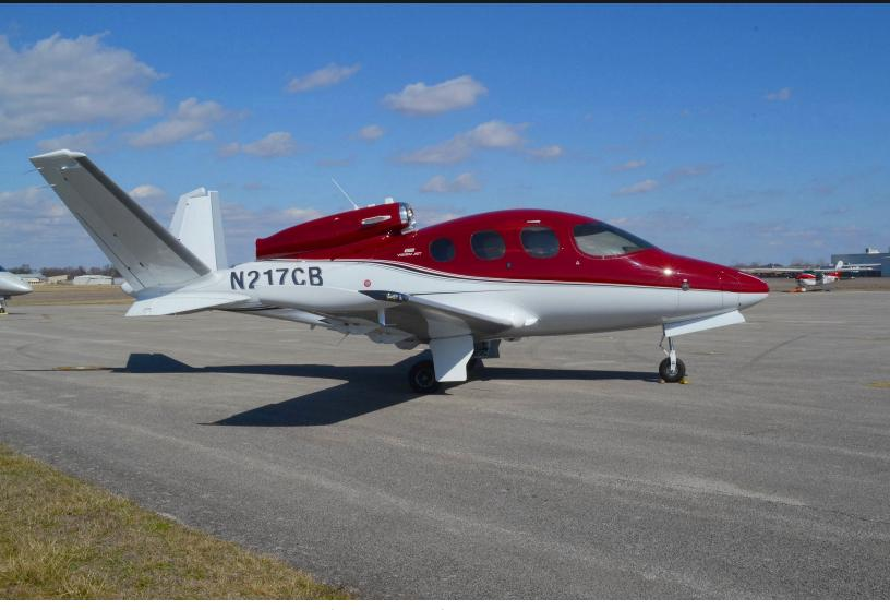
In 2018, the Vision Jet was awarded the Collier Trophy for the "greatest achievement in aeronautics in America". Powered by a Williams FJ33 turbofan, the all-carbon fiber, low-wing, seven-seat Vision SF50 is pressurized, cruises at 300 kn (560 km/h) and has a range of over 1,200 nmi (2,200 km). For emergency uses, it has a whole-airframe ballistic parachute system.
