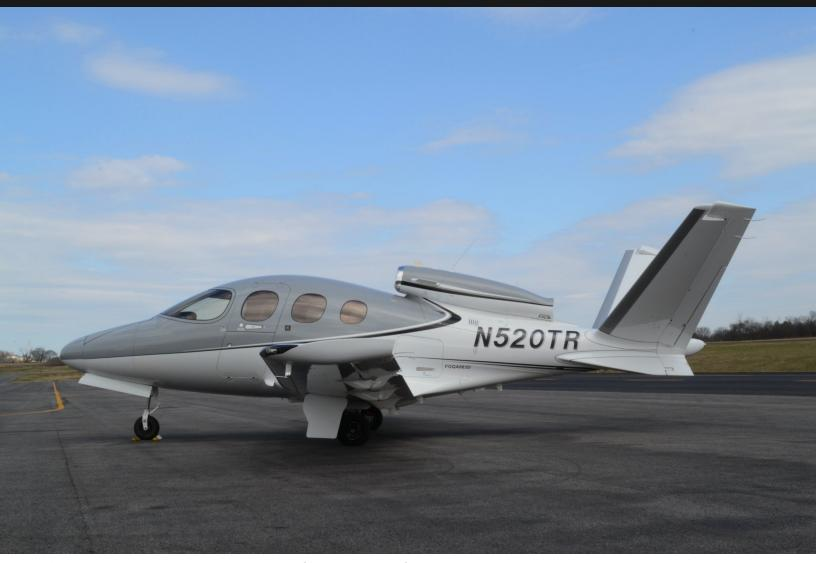
In 2018, the Vision Jet was awarded the Collier Trophy for the "greatest achievement in aeronautics in America". Powered by a Williams FJ33 turbofan, the all-carbon fiber, low-wing, seven-seat Vision SF50 is pressurized, cruises at 300 kn (560 km/h) and has a range of over 1,200 nmi (2,200 km). For emergency uses, it has a whole-airframe ballistic parachute system.
