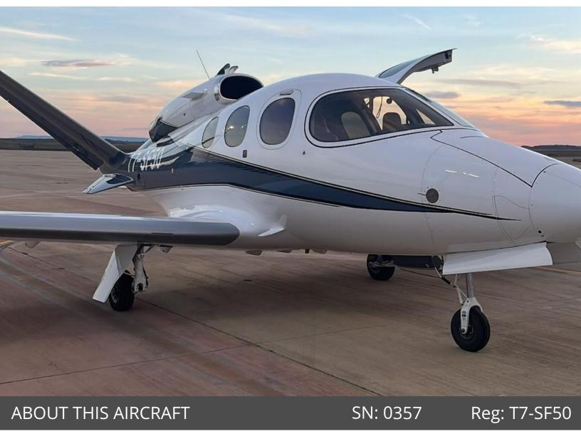
This beautiful, like-new Cirrus Vision SF50 G2+ has the optional emergency autoland system by Garmin, which the company introduced in October 2019. It initiates at the push of a button and is built into the G3000 integrated avionics. Cirrus calls the technology "Safe Return". This option is offered for \$170,000 including extra equipment, it allows landing on runways over 5,836 ft (1,779 m)
