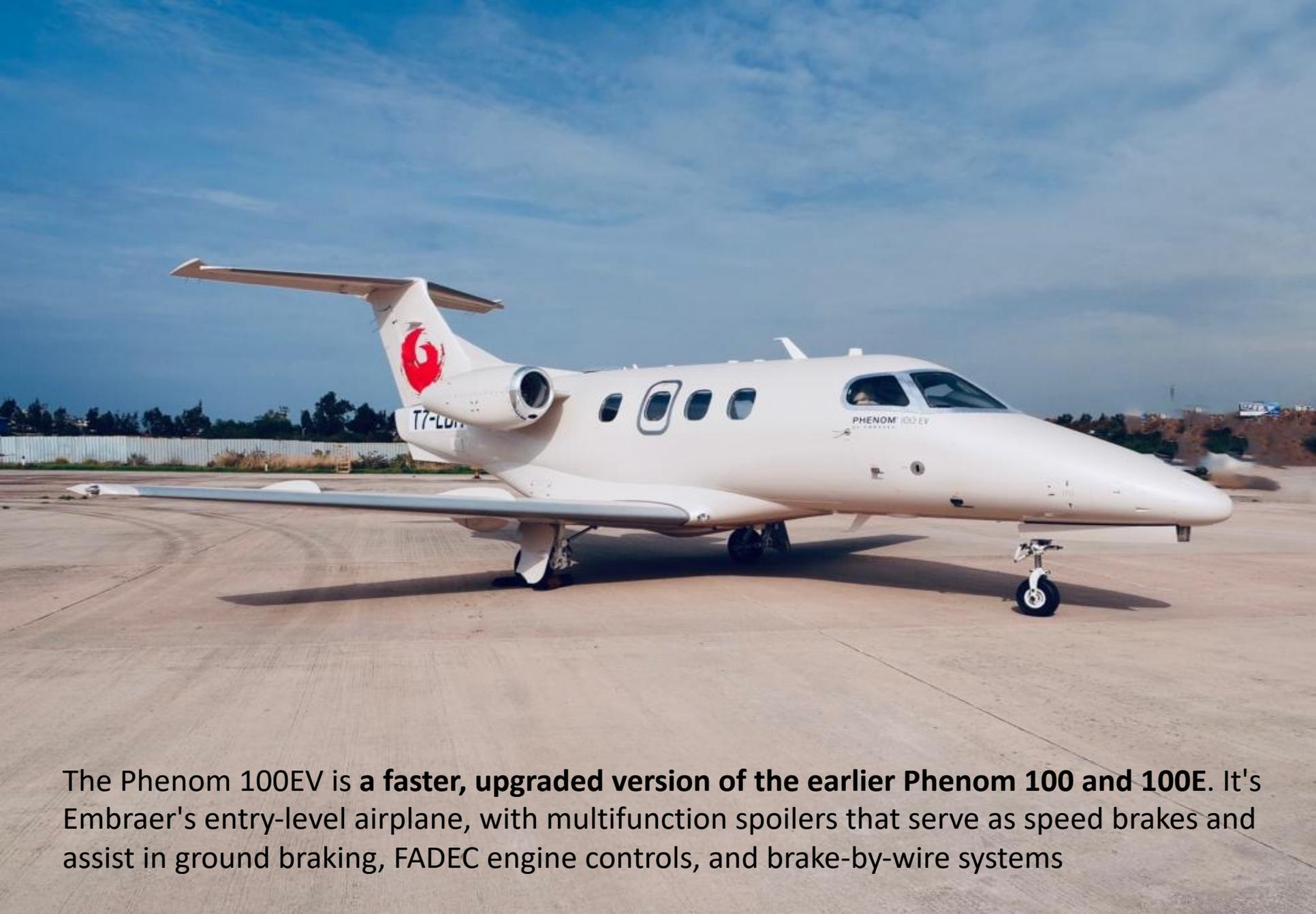
The Phenom 100EV is a **faster, upgraded version of the earlier Phenom 100 and 100E**. It's Embraer's entry-level airplane, with multifunction spoilers that serve as speed brakes and assist in ground braking, FADEC engine controls, and brake-by-wire systems
