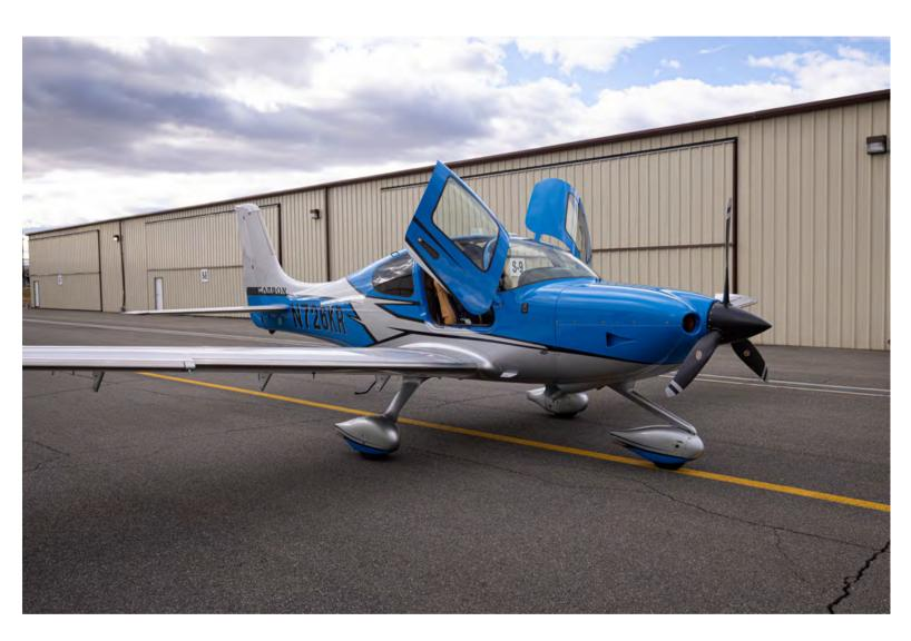
2018 G6 Cirrus SR22 with the Perspective+ Avionics Cockpit, all GTS packages including, All Digital 4-in 1-Standby Instrument, Enhanced Stability Protection (ESP), Synthetic Vision Technology (SVT), Enhanced Vision System (EVS), Air Conditioning, tubeless tires, and Beringer brakes
