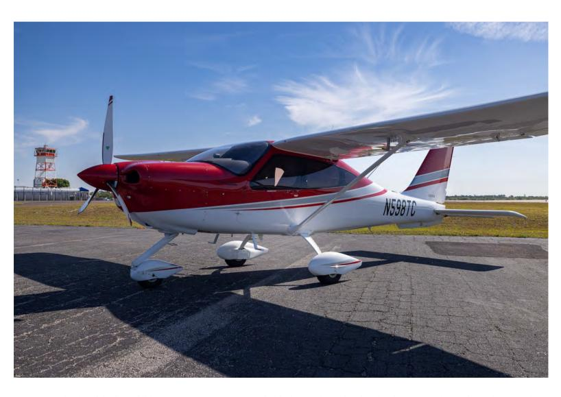
Lone Mountain Aircraft is pleased this Tecnam P2010 TDI equipped with the Continental Turbo Diesel CD-170 Engine and Garmin 1000Nxi Avionics Suite. This modern aircraft burns just 5.2 US Gal per hour with a fuel-tank capacity of 63 gallons giving you a range of 1000NM. The TDI engine grants excellent high-altitude performance with fast cruise above 140 KTAS at 10,000ft and ceiling up to 18,000ft.
