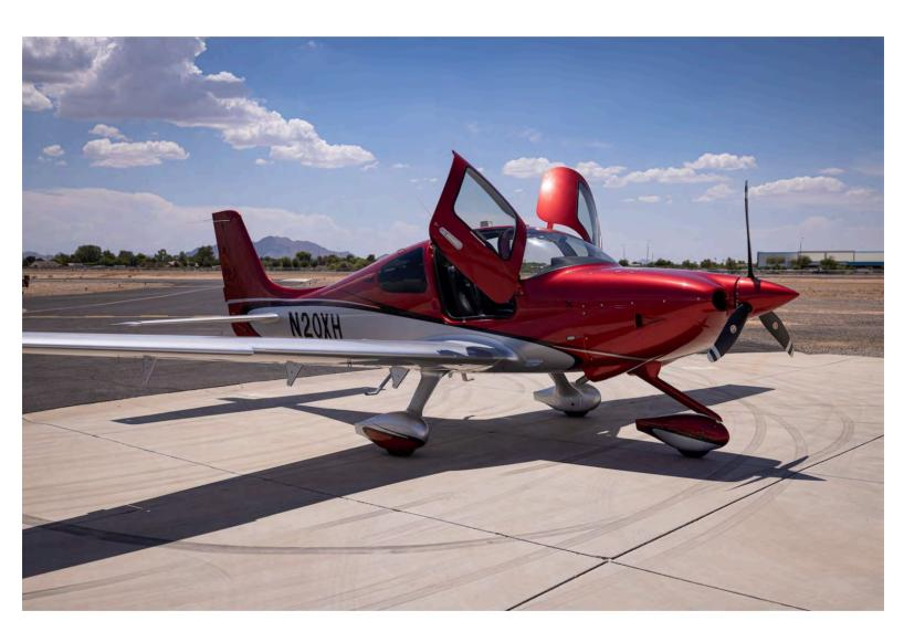
2025 Cirrus Premium SR20 G7 including Perspective+ Avionics Cockpit including 14" screens, GFC 700 Autopilot with Enhanced Stability Protection(ESP), Synthetic Vision Technology(SVT), Air Conditioning, tubeless tires, Beringer brakes, and more! Spinner to Tail warranty until March 24, 2030.
