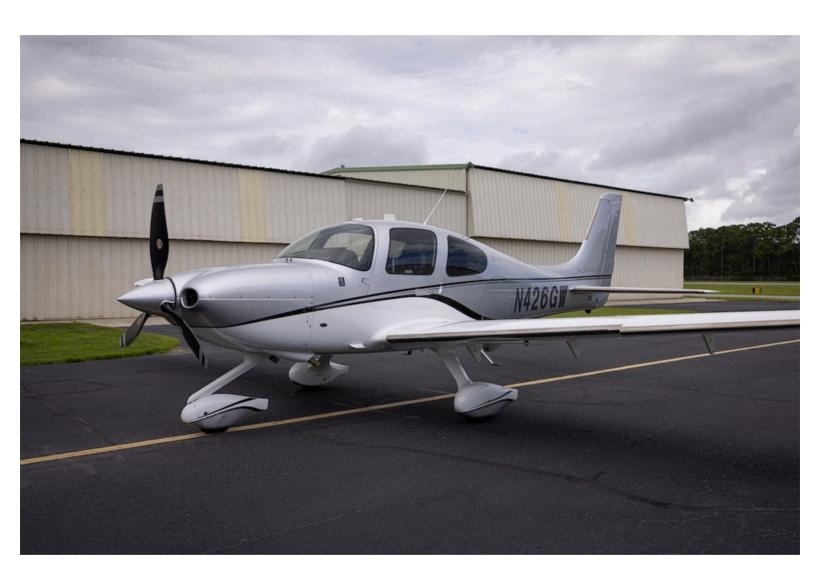
N426GW is a desirable configuration with the naturally aspirated 310 hp Continental IO550 and composite propeller, with all "GTS options". Equipped for Flight Into Known Icing along with Air Conditioning and much more.
