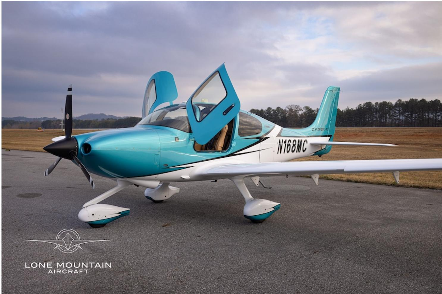
2023 Cirrus SR20 G6, including Perspective+ Avionics Cockpit including 12" screens, GFC 700 Autopilot with Enhanced Stability Protection(ESP), Synthetic Vision Technology(SVT), Air Conditioning, XM Weather, tubeless tires, Beringer brakes, and more! 5 Year Spinner to Tail Warranty through October 2028.
