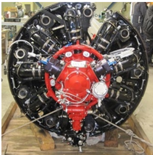
Engine following overhaul, before installation
